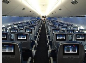
New seats, outlets, IFE, overhead bins
